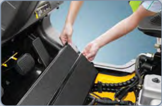
Tool-less floor plate for serviceability.
