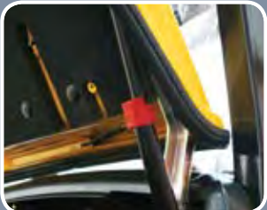
Automatic self locking gas spring Engine compartment hood is held safely open by a self locking gas spring.
