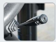
**Multi-Functional Switch** Integrated multi-functional switch lever enables the driver to operate lights and horn conveniently.
