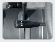
**Easy Control Direction Lever** Finger tip control of forward and reverse lever allows the operator to remain in control of equipment.
