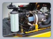
Easy change air cleaner The air filter is readily accessible for cleaning or replacement. (7inch Cyclone Type)
